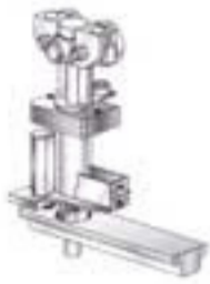
The traveling carriage with the current pick-up trolley ensures the power supply and data communication with the central control unit.
