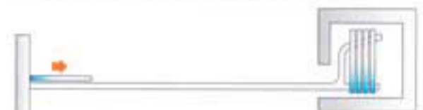
90° stacking area with sliding door
