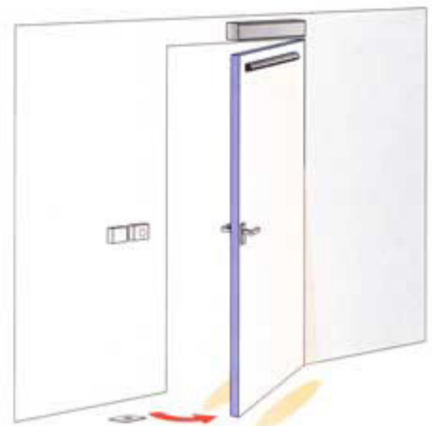
Safety sensors with configurable functions "Reverse" and "Stop" functions offer additional protection at the pinch points and in the event of oncoming traffic.
